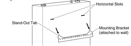
Figure 11 - Mounting Heater Onto Mounting Bracket
